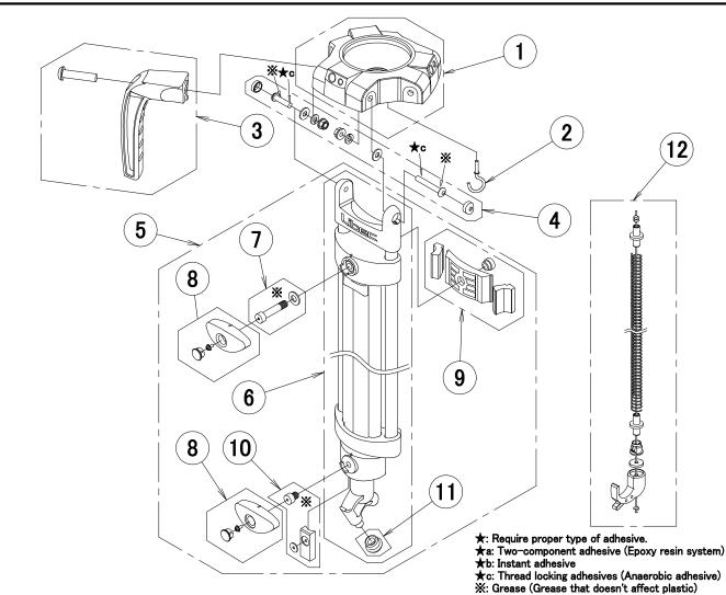
**QTY USED** PART No. No. **DESCRIPTION NOTE** PER PROD RT30RB-1 1 Leg base 1 2 RT30RB-2 Hook 1 3 RT30RB-3 Carrying handle 1 4 RT30RB-4 3 Leg screw set 5 RT30RB-5 Leg assembly 3 3 6 RT30RB-6 Leg semi assembly 7 RT30RB-7 Upper lock bolt 3 8 RT30RB-8 Leg lock knob 6 9 RT30RB-9 Leg stopper (Female) 3 10 RT30RB-10 Lower lock bolt 3 11 RT30RB-11 Spike cap ×3 pcs 1 12 RT30RB-12 Binding strap 1
