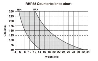
\*When the innerspring is set to maximum strength, the tilt angle is limited to +/-40 degrees.
